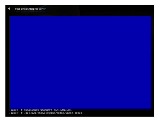
Now we will execute the VHCS2 setup file. Type the following into the shell: "/srv/www/vhcs2/engine/setup/vhcs2-setup"
